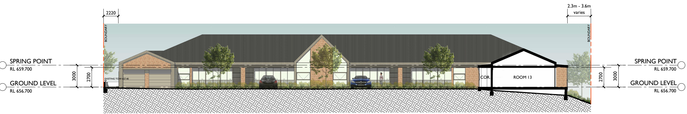
INTERNAL NORTH ELEVATION / SECTION F-F
