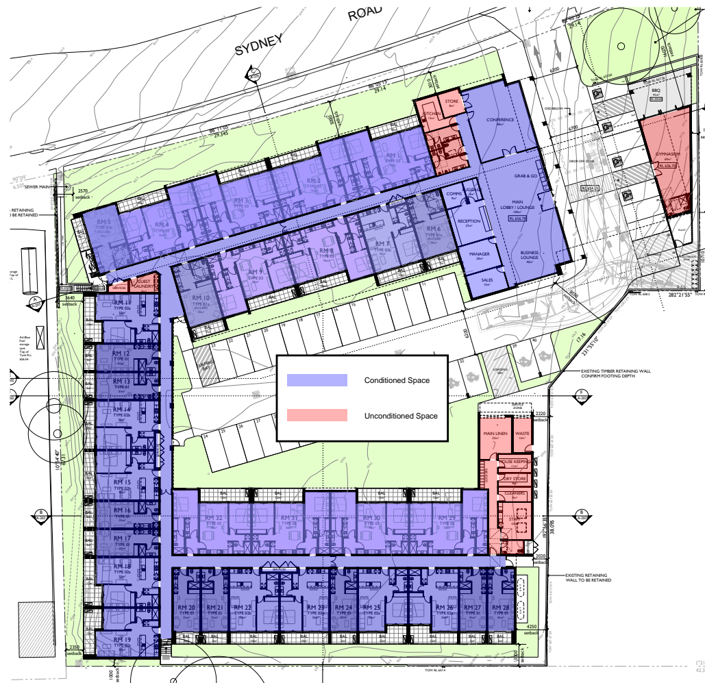
Figure 1 – Ground floor envelope
