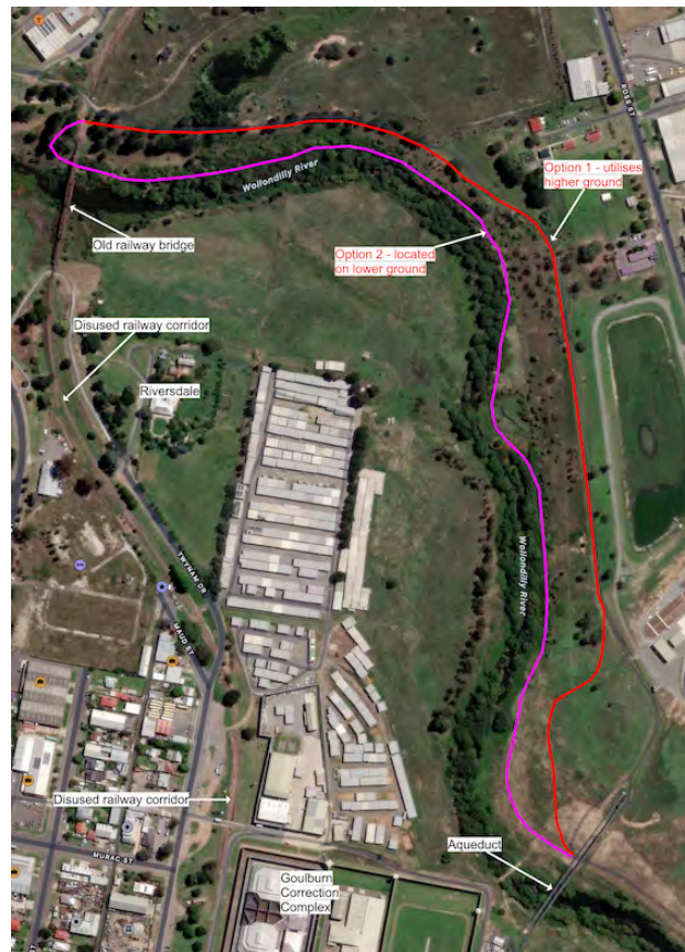
Figure 1: Route options – connecting the Goulburn aqueduct to the Wollondilly River rail bridge
