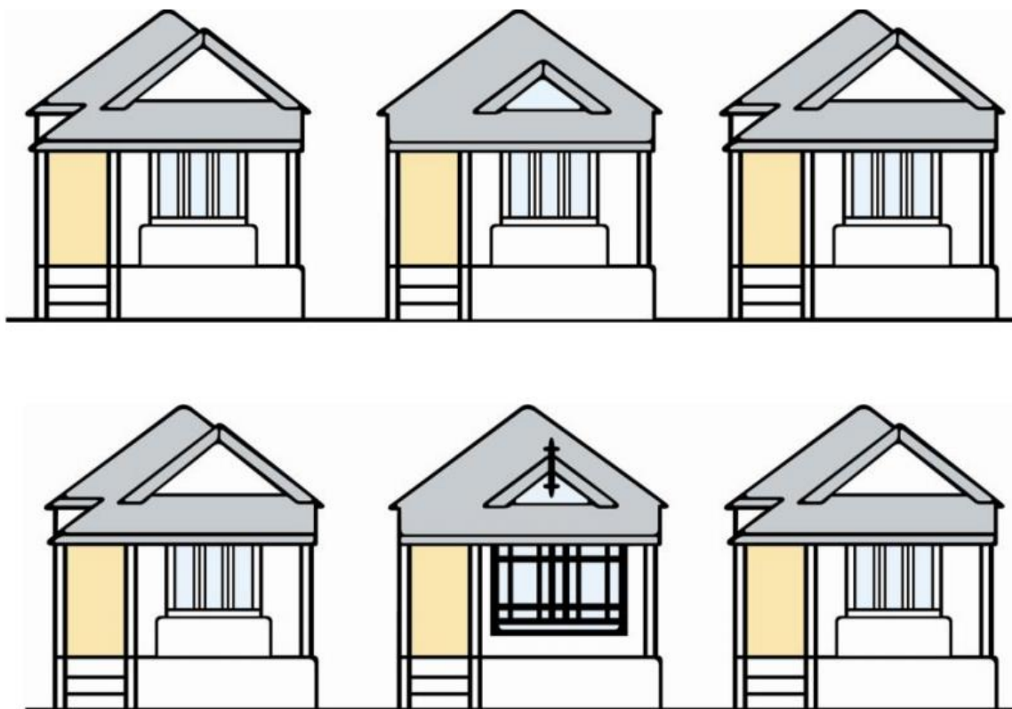
Figure 3.8: This example does NOT respect the massing and form of surrounding buildings
