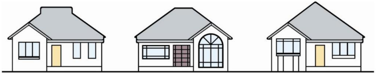
Figure 3.12: Existing pattern of simple cottages with vertically proportioned doors and windows versus new development that does not respect the existing pattern, with uncharacteristic arched window and double leaf door.
