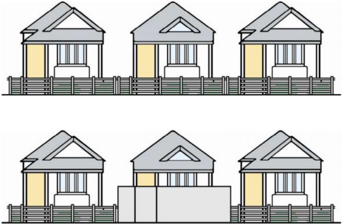
Figure 3.16: High and solid fencing destroys the harmony of the streetscape and prevents views of the dwelling and front garden
