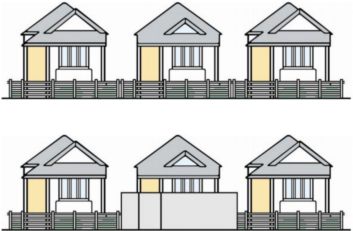
Figure 3.16: High and solid fencing destroys the harmony of the streetscape and prevents views of the dwelling and front garden
