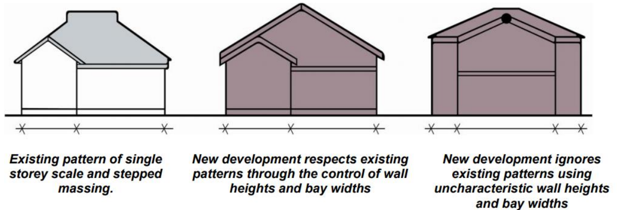
Figure 3.14: Example of new development not respecting pattern of existing façades
