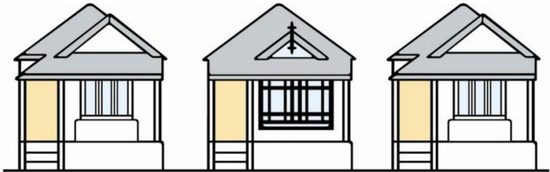
Figure 3.9: Existing pattern of simple cottages versus new development that does not respect the existing pattern by selecting windows that are out of proportion and adding an over-scaled finial to the gable.
