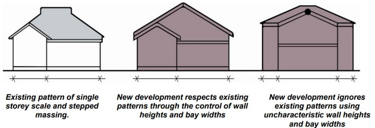
Figure 3.14: Example of new development not respecting pattern of existing façades
