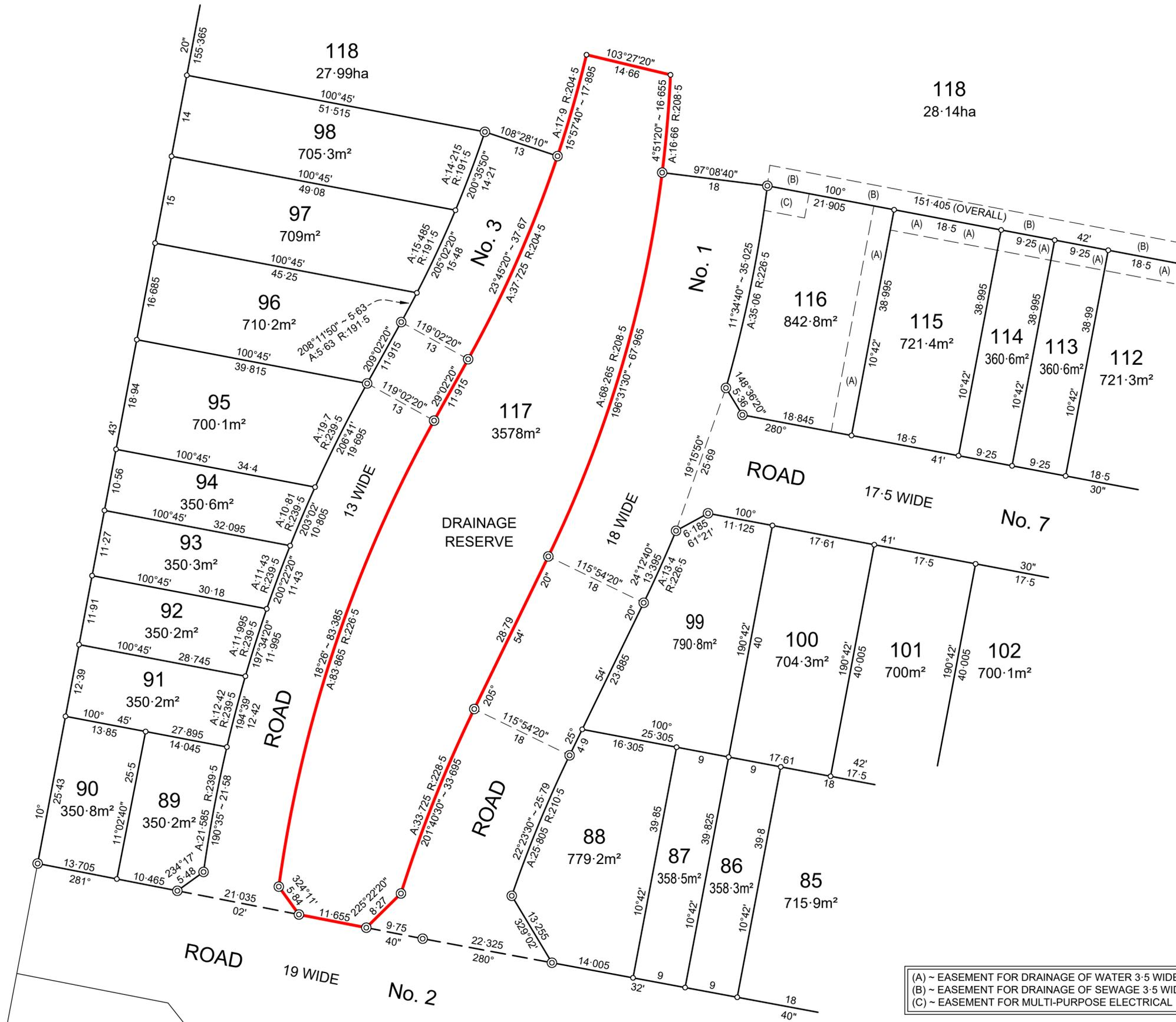
(A) ~ EASEMENT FOR DRAINAGE OF WATER 3.5 WIDE ~ (No. 1)
