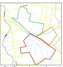
The most significantly affected areas are those identified as Flood Planning Constraint Category 1 (red) and 2 (blue) where flood inundation is most frequent and severe, indicating where development should be avoided. These areas are proposed to be zoned as C2 Environmental Conservation where most development types are prohibited.
