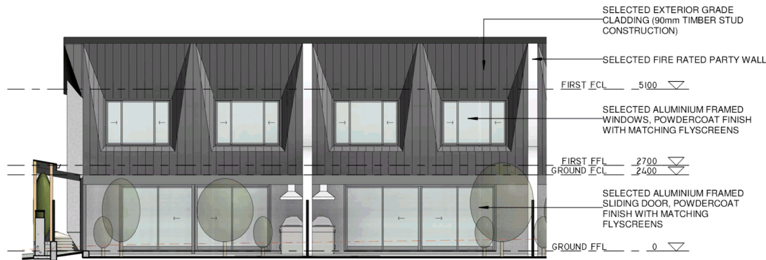
3 DETAIL NORTH ELEVATION 1 : 100 @ A3
