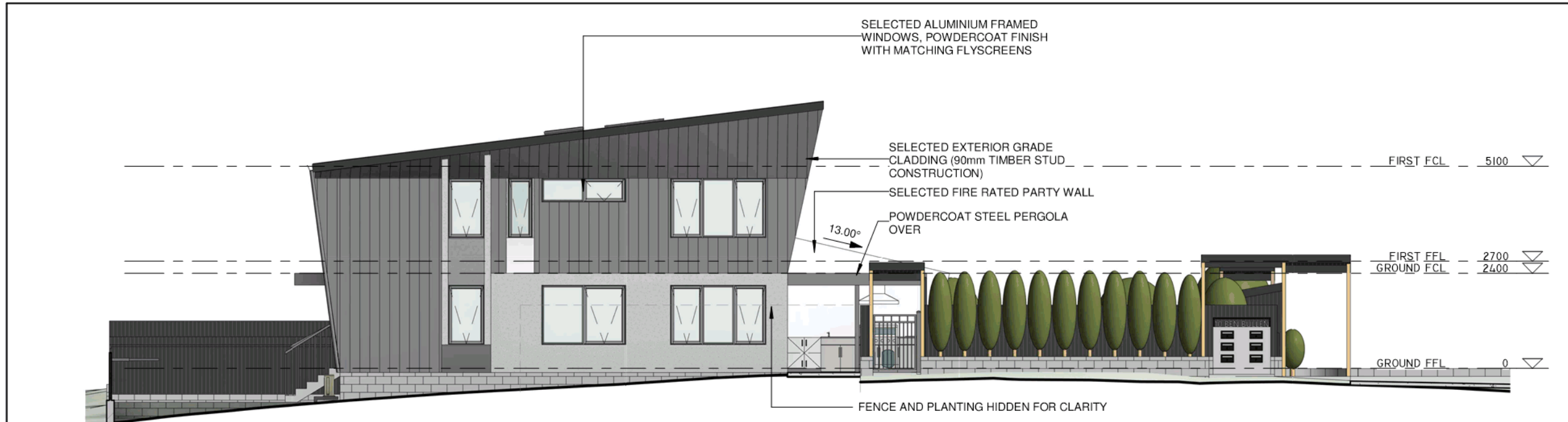
1 DETAIL EAST ELEVATION 1 : 100 @ A3
