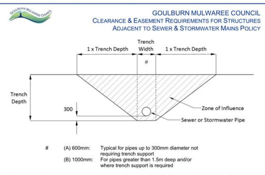
The design of a structure's footings can be configured to transfer loads outside the zone of influence to allow building within the zone. Structures are only permitted within the zone of influence (but outside the minimum clearance requirements) under the following conditions:
