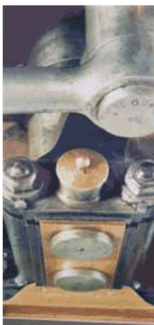
Before – oil well lid in place
